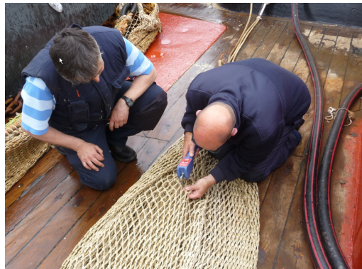
Figure 3 typical mesh size measurement with objective mesh gauge (OMEGA)
